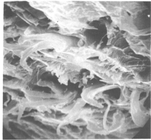
Figure 11 Fractograph of the coir fibre showing pull-out of the cells and collapse of the cell walls ( \times 1375 ).
